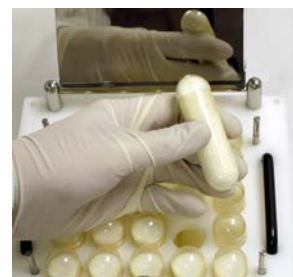
15. Remove capsules from the Caps Tray. You now have fully locked and filled capsules. With practice you can fill 400+ capsules per hour.
