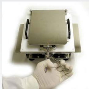
5. Pull the Cam Handle about 60-80° to secure capsules in the Filler. Capsules should be held firmly but not squeezed to an oval shape.
