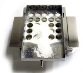
8. Place the Powder Tray on the Filler with the powder reservoir towards operator. Pour pre-measured powder onto Filler.
