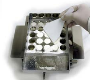
9. Spread powder evenly using the Powder Spreader. Push excess powder onto Powder Tray reservoir.
