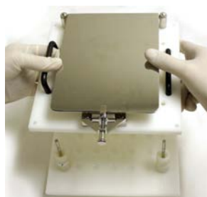
13. Place the Caps Tray containing reassembled capsules on Locking Base by placing it over the Locating Pins.
