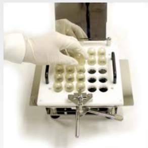
4. Place the Caps Tray onto the Filler. Load the capsules into the Caps Tray (longer narrower side first). Close the Locking Plate & Clamp to secure.
