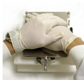
14. Lock the capsules by applying pressure with both hands (palms) as shown.
