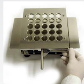
7. Release Cam Handle to drop capsule bodies into the Filler. Gently pat down capsules.
