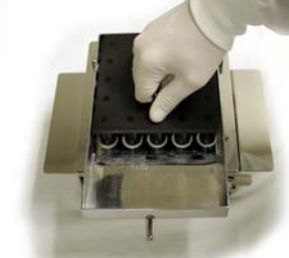
10. Use Tamper to pack powder. Repeat spreading and tamping as necessary. Remove Powder Tray when done
