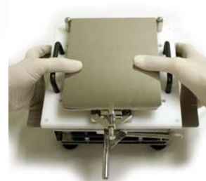
11. Place Caps Tray onto the Filler. Reassemble capsules by pressing on the Locking Plate while lifting Lifting Plate. Do not try to Lock on Filler .
