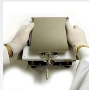
6. Separate the capsules by pressing thumbs down on Caps Tray Handles while evenly lifting up Caps Tray. Set aside Caps Tray.
